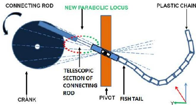
**Figure 5: Connecting ROD Showing Telescopic Section Attached to Crank.**
