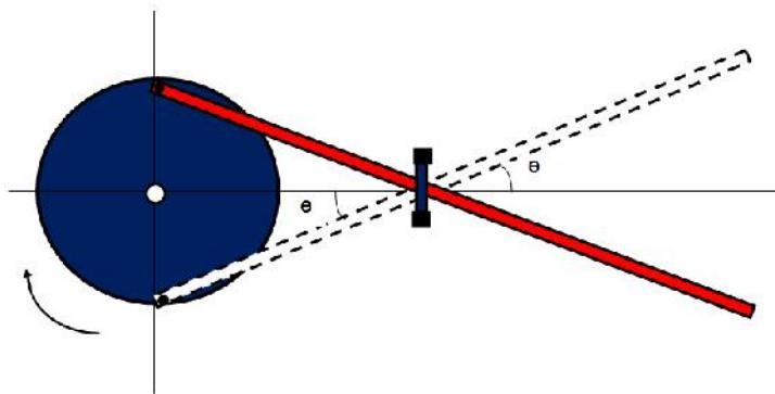
**Figure 3: Maximum Swing Angle of a Modified Crank and Connecting Rod Assemble**
