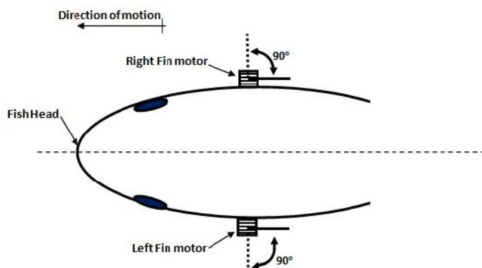
**Figure 6: Diagram of Fish Upper Head Region Showing Motion of the Pectoral fin DC Motors.**
