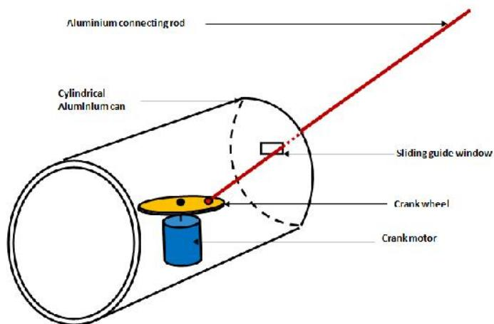
**Figure 7: Fish Core, Crank Motor, Crank Wheel and Connecting rod Assembly.**
