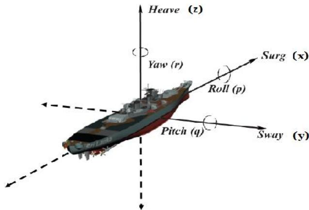
**Figure 1: Description of 6 Degrees of Freedom of a Ship.**
