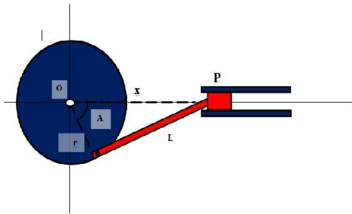
**Figure 2: Typical Crank, Connecting Rod, Piston Assembly**
