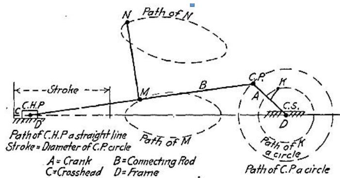
**Figure 4: Ellipse Produced by Point M on a Connecting Rod for a Typical Crank- Connecting Rod Mechanism.**
